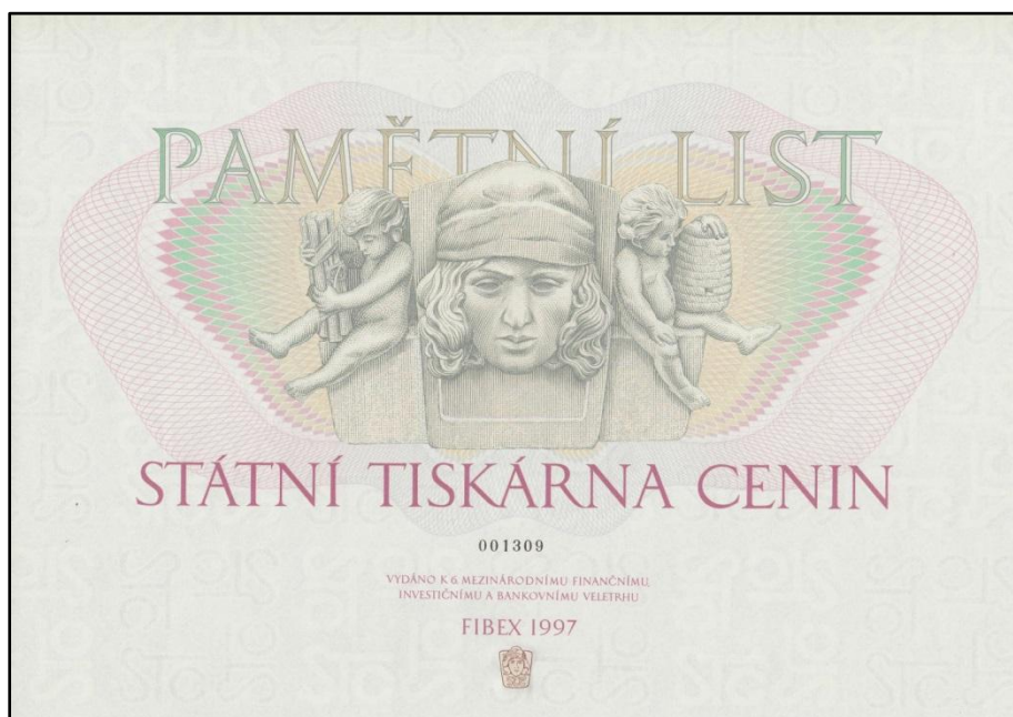
Figure 8 - STC, 1997 Security paper with watermark. Gravure printing - engraving (logo under the text "FIBEX 1997"), offset printing
